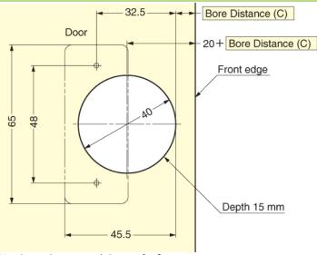
Use Size 5 Countersunk Screws for fixing.
